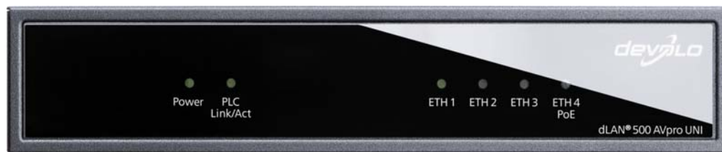
Fig. 4: LEDs on the front of the dLAN 500 AVpro UNI
